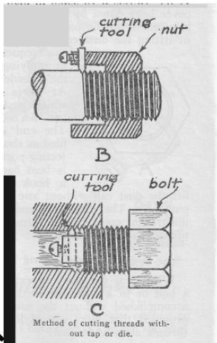
At (Fig A) is an end view of the nut with the cutting tool in place. It will be seen that the cutting edge is in line with the center of the nut. The threading is accomplished in the same manner as with a die. As all the cutting is done by the single cutting edge, it is advisable to take three or four cuts, lowering the tool after each cut.
