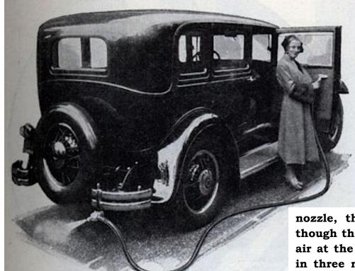
Using the exhaust gas of the automobile to clean the upholstery is the accomplishment of a recently invented device. An aluminum attachment is fastened to the exhaust pipe and the engine is allowed to As the exhaust idle. gas passes through this device suction is created at the inlet hole. Collected by a
