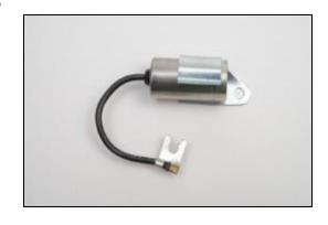
just loosen the coil terminal nut, attach the "pig tail" clip, tighten terminal nut again and be merrily on your way. If you should wish to use this modification, the condenser will serve for years as it is located away from intense heat of the motor. Heat is the worst enemy of the stock Model "A" Ford condenser.
