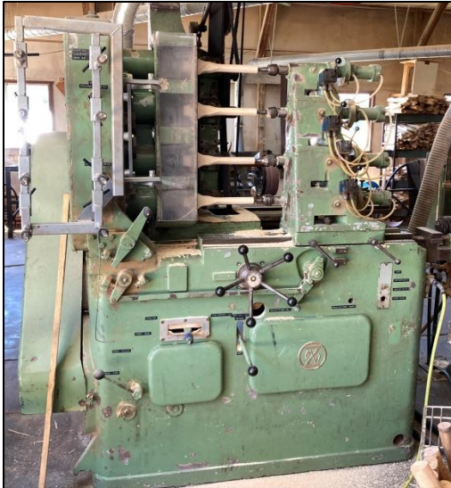
The wooden spoke lathe turns four spokes at the same time.
