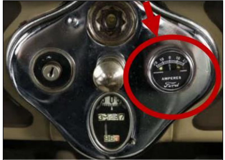
1928 - 1930 Ford Model “A” instrument panel with the ammeter location highlighted.
