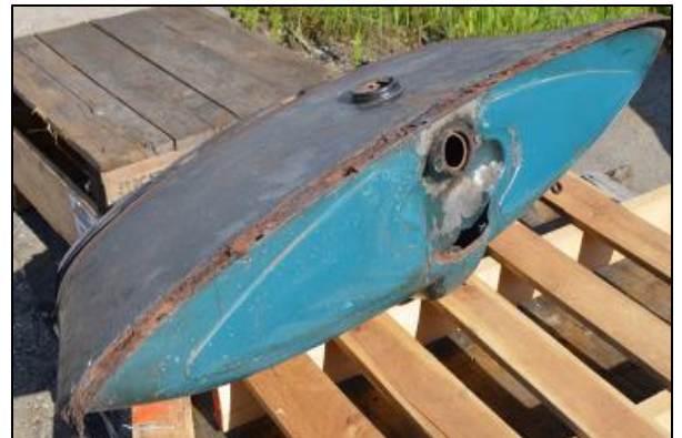
The gas tank sitting in Wisconsin being prepared for an acid bath.
