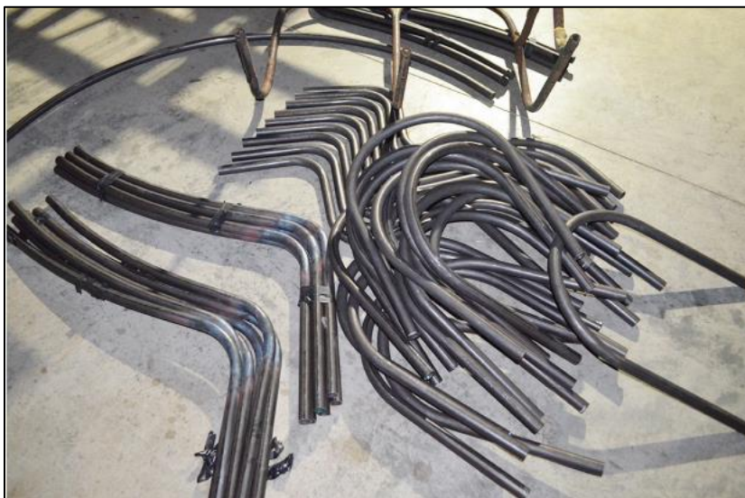
The new bus seat frames being formed at Chicago Tube & Iron.
