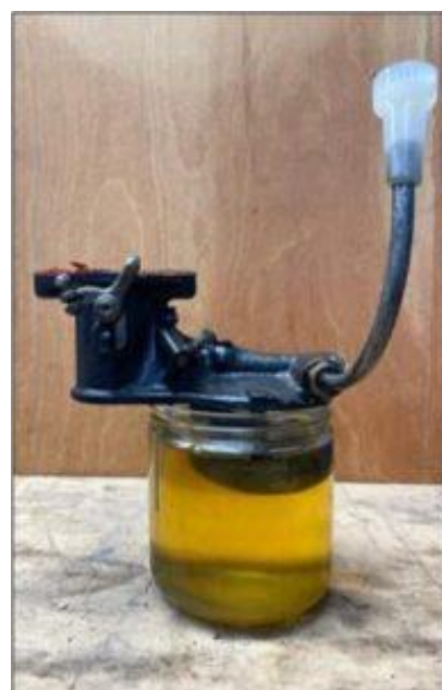
Eric Shogren's float valve tester.
