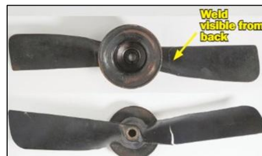
2. Weld location and failure area.
