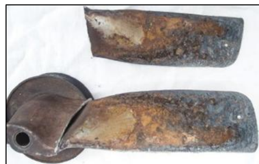
1. Inside of an original hollow blade.
